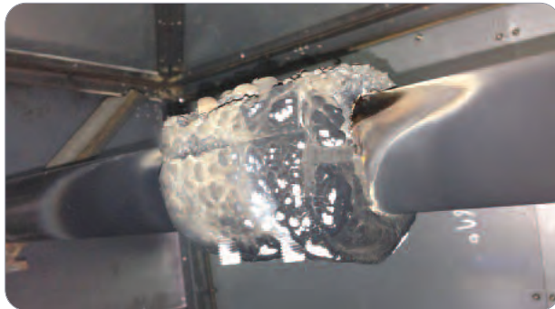
▲ The product after completion of the test with normal pressure being maintained at over 800°C
