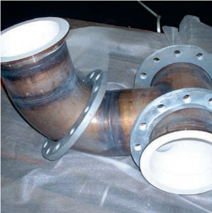
POWDER COATED PIPELINE
