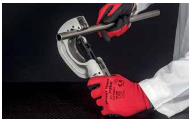
Taglio del tubo / Cutting the pipe to length
